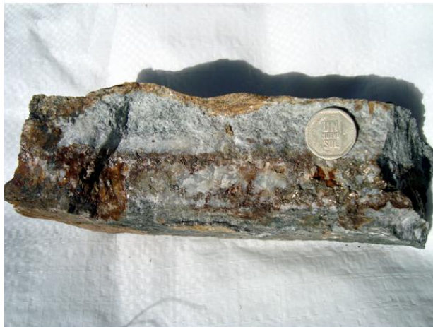
Figure 3.21: sample of quartz vein associated with pyrite, subordinate chalcopryrite and iron oxides
