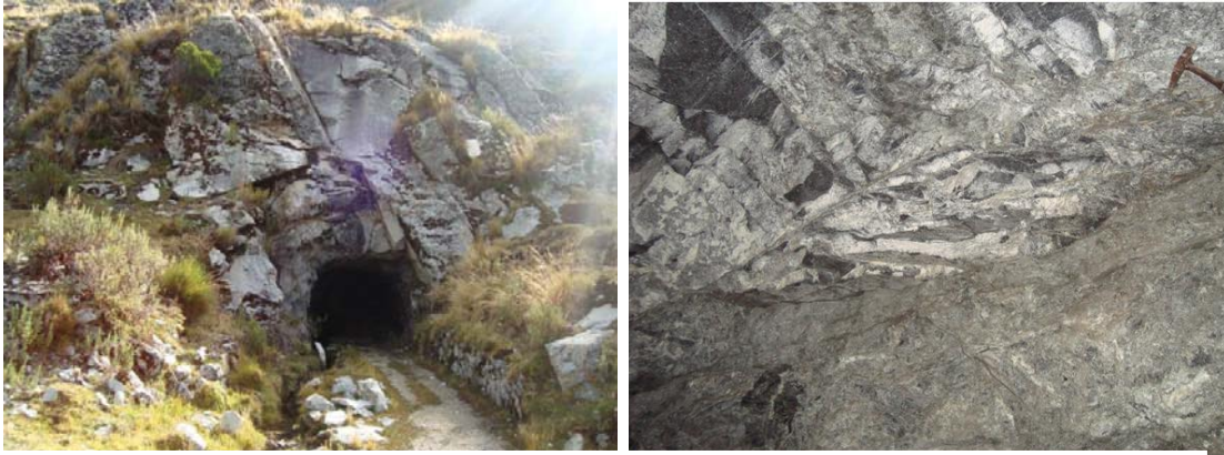
Photo 3.13: Yuringa mine of intrusive rocks (tonalite). Note the fracture rate associated with normal faults. Informal mining work.
