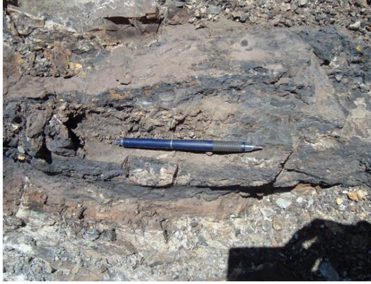
Photo 3.5: brecciated structure with oxides of manganese and iron oxides, hematite-goethite, limonite, pyrolusite and marbled limestone cutting direction N70W. Note the mining work.
