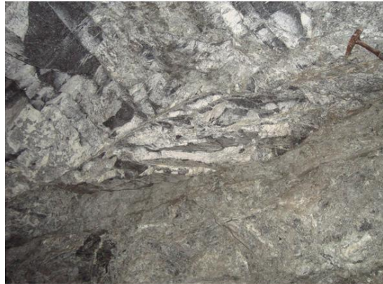
Photo 3.13: Yuringa mine of intrusive rocks (tonalite). Note the fracture rate associated with normal faults. Informal mining work.
