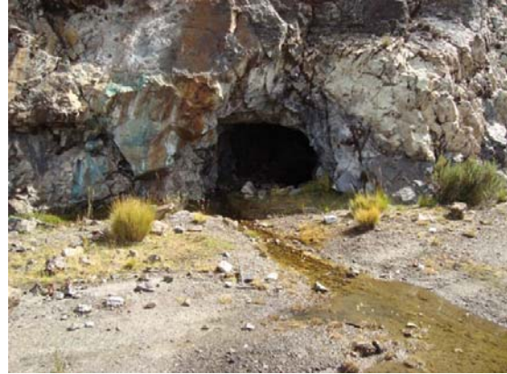
Photo 3.17: Pit in old work of mine showing fault plane with chalcocite, molybdenite and copper oxides.
