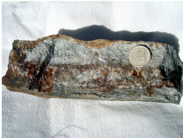
Figure 3.21: sample of quartz vein associated with pyrite, subordinate chalcopyrite and iron oxides
