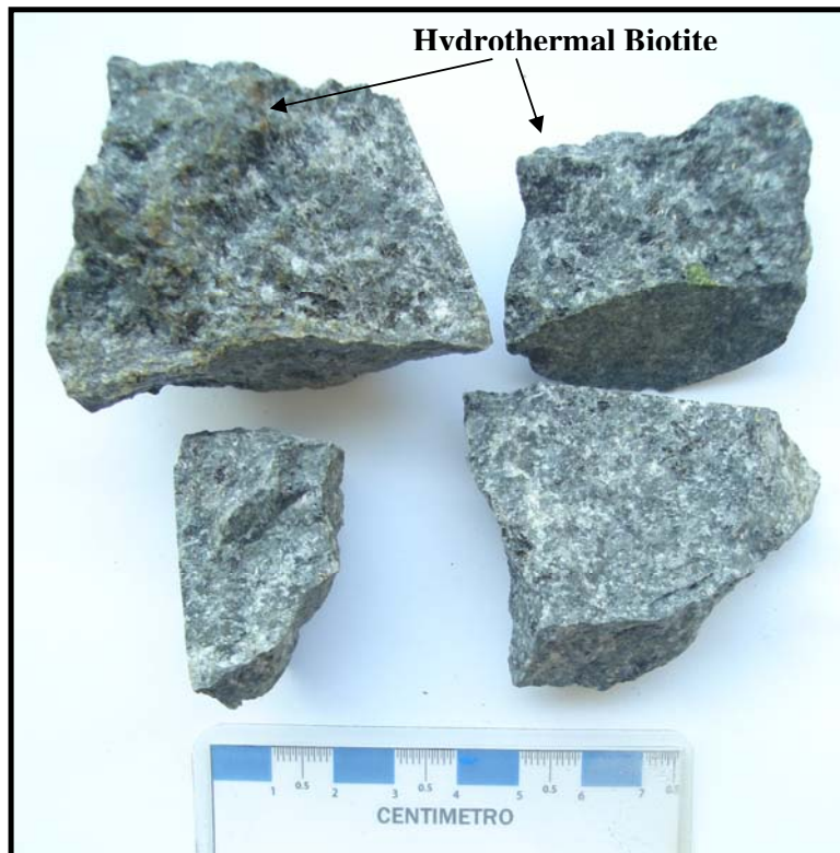
Foto N° 5.6.- Hydrothermal biotite in small grains associated with potassic alteration and type B veins (Azulccaca Porphyry).
