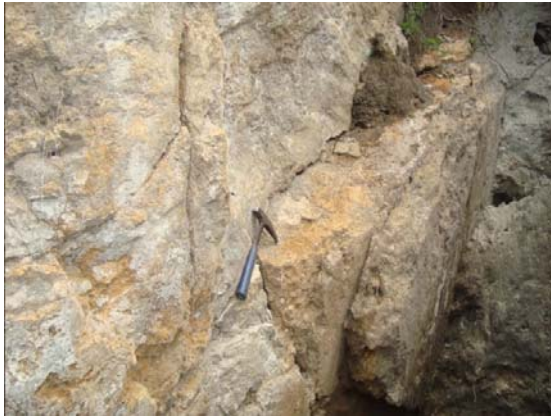
Photo 3.11: Structure with iron oxides hematite-goethite-limonite N55W course cutting limestone. Informal mining work.
