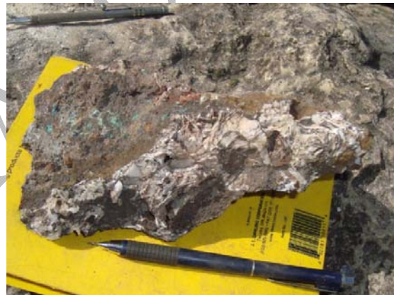
Photo 3.15: dextral fault plane. Note the kinematic structures indicating the direction of motion. Inside the mine.
