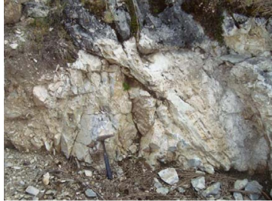
Photo 3.9: brecciated structure with iron oxides hematite-goethite-limonite N55W course cutting limestone.
