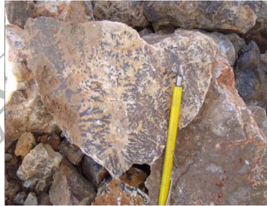
Photo 3.7: brecciated structure with oxides of manganese and iron oxides hematite-goethite-limonite. Direction N70W. Esperanza pit.
