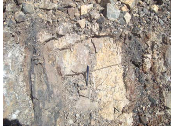
Photo 3.5: brecciated structure with oxides of manganese and iron oxides, hematite-goethite, limonite, pyrolusite and marbled limestone cutting direction N70W. Note the mining work.
