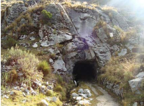
Photo 3.13: Yuringa mine of intrusive rocks (tonalite). Note the fracture rate associated with normal faults. Informal mining work.
