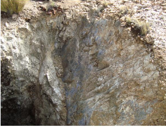
Photo 3.17: Pit in old work of mine showing fault plane with chalcocite, molybdenite and copper oxides.
