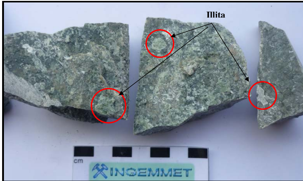
Photo N° 5.7.- Disregarded sample for isotopic studies where it is observed illite minerals, who had been confused by the chlorite. (Ccarayoc Porphyry).
